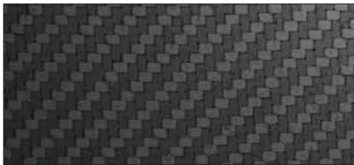
Above: Close-up of 2 x 2 carbon fiber weave. This is genuine carbon fiber, not a cosmetic dress-up with a carbon fiber pattern!
