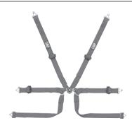
This 2x2 harness has a pull-up lap belt with bolt-in end plates sewn in. The sub straps include bolt-in end plates that can convert to wrap-mount. The shoulder straps have bolt-in end plates sewn in or a sewn loop to accept a cross bolt. FIA 8853/2016 approved. Black or Red.
