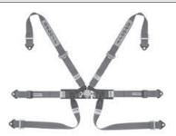
These 2x2 harness have a pull-up lap belt with a 3" wide spreader pad behind the buckle. Instead of metal D-rings, the sub straps pass through fabric loops sewn on the lap belt. The shoulder straps and sub straps include bolt-in end plates that can convert to wrap mount. The lap belt has bolt-in end plates sewn in. FIA 8853/2016 approved. Black, Blue, or Red.
