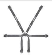
To reduce weight and bulk, this 2x2 harness has no quick-adjusters on the lap belt. Length is set on installation. Instead of metal D-rings, the sub straps pass through fabric loops sewn on the lap belt. All 6 belts include bolt-in end plates that can convert to wrap mount. FIA 8853/2016 approved. Black or Red.
