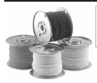
This is an excellent quality stranded wire. The thick wall cross-linked SXL insulation is rated for 125°C and is resistant to oil, gas, grease, and acid.
