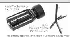
sures caster and camber with three bubble levels. Bright markings and separate positive and negative scales reduce errors and confusion. Magnetic adapter (included) makes it easy to use with most steel wheels, hubs, or discs. Other adapters (such as the folding Quick Set adapter) are available separately. Case included.
