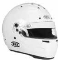
The **RS7** is based on the advanced Bell HP7 helmet currently used in F1. A total of 14 inlet and exhaust vents provide maximum cooling. The shield pivot shape is designed to minimize wind noise at speed. Includes one clear dual-pane anti-fog shield (Bell SE07 size). Snell SA2015 and FIA 8859-2015 approved. Available in white or flat black. Specify size: 7 1/8 through 7 5/8.
