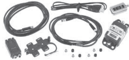
X2 Direct-Wire Transponder Kit, Part No. 5001-51x Clockwise from lower left: X2 RaceKey Mount, power cable, USB cable, X2 RaceKey, X2 Transponder, permanent-mount hardware, quick-release mount bracket. The cable in the center connects the X2 Transponder to the X2 RaceKey Mount in the car.
