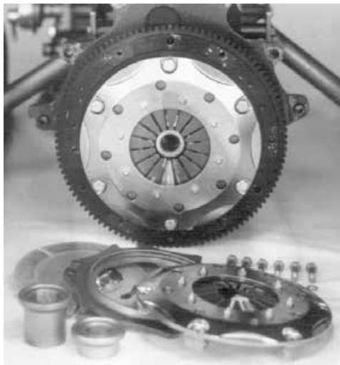
Tilton OT2 Clutch mounted on Ford 2.0L engine (Part No. 173-15-Gray Clutch Assembly with Part No. 173-16-OT2 Disc)
