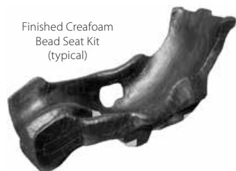
Finished Creafoam Bead Seat Kit (typical) The seat insert above was created for a sports racer using an X-Large (30 Gallon) kit. It was covered using 2 rolls of Gaffer's Tape.
