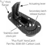
Part No. 3038-001-Carbon Look (sold in pairs; one shown) The **AeroCatch** is a new twist on hood pins. Hidden inside the aerodynamic thermoplastic housing is a stainless steel clevis pin which engages an anodized high-strength aluminum hood pin. The entire mechanism is fully enclosed and protected.
