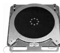
**Intercomp Mechanical Turn Plates** have precise CNC machined numbers to indicate from -35 to +35 degrees. Three levels of case-hardened roller bearings allow free movement in X and Y directions as well as rotation. The high-friction top surface eliminates tire slippage for accurate measurements. Can be zeroed with car in place. Plate measures 13" x 15" x 1.5" high. 2000 pound capacity per plate.
