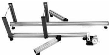
**ART Laser Toe Gauge** This professional gauge uses laser precision to measure toe down to one minute of a degree. Requires only 12mm of ground clearance, so aerodynamic devices can stay in place. Weighs less than 20 pounds. Easy for one person to set up and use.
