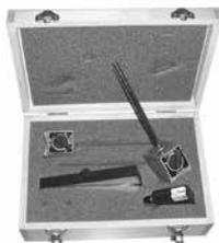
**ART Laser Bump Steer Gauge** Laser accuracy is now available in a bump steer gauge! Using a simple laser, mirror, graph paper, magnetic bases, and a shutter, you can now measure bump steer with an accuracy up to millionths of an inch if desired. It doesn't bolt to the hub, so it can be used on a wide variety of hub types. The lack of a bulky frame also makes it easily portable. Easy to use, yet accurate enough for professionals. Includes padded wooden carrying case.
