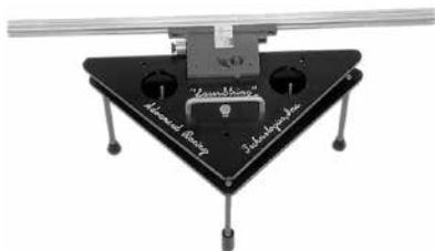
**ART Laser Strings** These extremely versatile tools shoot a laser plane (not a beam) along the side of the car. One person can check frame straightness, rear axle alignment, and 4-wheel toe. You can also use them to align graphics, set up scales, and for many other applications. Choose Single (one plane) or Triple (3 parallel planes).
