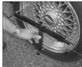
The **Dream Stick by ART** is an innovative tool used to measure toe with a string, or with any ART Laser String product. Dual scales read the distance from the string to both the front and back of the rim at the same time. Adjusts to fit wheels from 12" to 20" diameter. Locates on the rim using three contact points to ensure the scales are perpendicular to the rim. Scales have both English and Metric markings.
