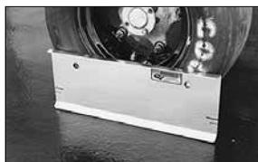
The **Longacre Toe Plate** kit is one of the quickest and simplest ways for you to measure total toe. Just rest one plate on the side of each tire and use measuring tapes to find your setting. Magnets help keep the tapes in place on the plates. Kit includes 2 toe plates and 2 tape measures.
