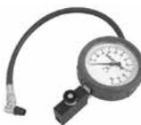
Why waste time juggling a tire pressure gauge and a filler chuck? This combination gauge makes the job quicker and easier. Just hold the angled chuck on the tire and read the gauge. Press the trigger to fill the tire, or press the bleed valve button to let air out. The oversized 4" gauge reads 0-60 psi in 1 psi increments. Female 1/4 NPT inlet threads requires male air hose fitting (not included).
