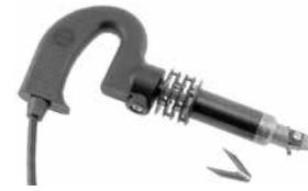
Our deluxe 250 watt, 120 volt pistol grip grooving iron has a solid brass head that preheats the rubber in front of the cutting blade, making it fast and easy to cut grooves and maintain accurate control. Includes a .215" wide cutting head and 12 matching cutting blades. Extra heads and blades in this width as well as a wider, .375" size are also available.
