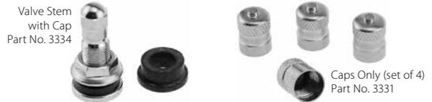
These chrome-plated valve stems fit most cast and modular wheels. The nut is on the outside so you can check tightness without dismounting the tire. Length is approximately 1" to 1.2" above the rim depending on the rim thickness. Rubber bushings included for both large and small rim holes.
