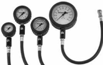
**Intercomp Deluxe Air Pressure Gauges** The most durable and shock resistant in the industry. Has only four moving parts in their patented internal mechanism vs. 14 or more in other gauges. Fewer moving parts means greater reliability. All have 17" Goodyear hose and thumb-operated bleeder with a swivel nozzle. 0-15 x 1/2 psi; 0-30 and 0-60 x 1 psi gauges; 2" standard, 2 1/2" liquid filled and 2 1/2" and 4" glow in the dark offer a great selection at an exceptional value.
