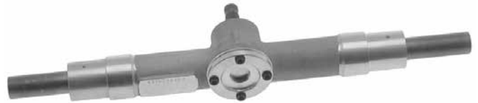
Stock Steering Rack, Part No. 1802 Dimensions of Stock Steering Rack: • 18" Rack Bar Length • 13" Housing Length • 10" Between Mounting Shoulders • 1.5" Housing Diameter at Mounting Bosses • 1/2-20 UNF Female Threads on Rack Bar Ends
