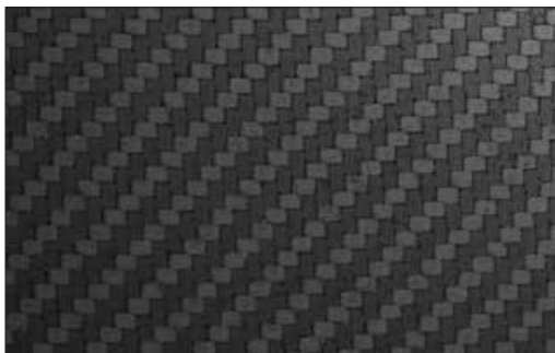
Above: Close-up of 2 x 2 carbon fiber weave. This is genuine carbon fiber, not a cosmetic dress-up with a carbon fiber pattern!
