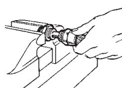
**Step 3** Lubricate nipple and socket threads with Aeroquip Assembly Lube (Part No. 3315) or an equivalent petroleum lubricant. Lubricants containing chloride are not recommended. (Stainless steel hose ends should use a moly-based lubricant such as Molykote G.) Hold the nipple with hex in the vise. Push hose over nipple with twisting motion until seated against nipple chamfer. Push socket forward and start threading of socket to nipple.
