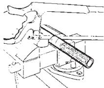
**Step 1** Wrap hose with glass filament strapping tape at cut-off point and cut squarely through tape to length using an Aeroquip Cut-off machine or a very fine tooth hacksaw. Remove tape and trim loose wires flush with tube. Remove burrs on bore of tube with a knife. Clean the hose bore.
