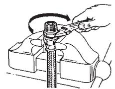
**Step 4** Tighten hex until clearance with socket hex is 1/32 inch or less. Tighten further to align corners of nipple and socket hexes. **CLEAN, PROOF TEST TO TWICE OPERATING PRESSURE, AND INSPECT ALL ASSEMBLIES.**
