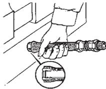
**Step 2** Push the sleeve over the end of the tube and under the wire braid by hand. Push the hose end against a flat surface until the tube butts against the inside shoulder of the sleeve. Set the sleeve barbs into the PTFE tube by pushing a round nose tapered punch into the end of the tube.
