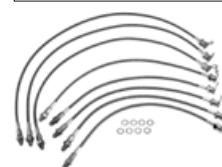
These hoses are constructed with the proper lengths, hose ends and adapters to allow easy retrofitting on a Spec Racer. SCCA legal.
