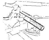
**Step 1.** Cut the hose square to length using a Cut-off Machine or a very fine tooth hack-saw. To minimize wire braid flare out, wrap hose with glass filament strapping tape.
