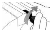
**Step 4.** Push the hose firmly onto the thread while rotating the hose. Keep turning the hose until the first three to four threads have engaged.
