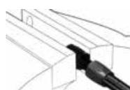
**Step 3.** Hold the fitting in a vice with smooth or soft jaws, and lubricate the threads with a light oil.
