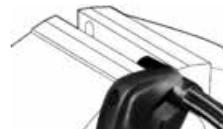
**Step 5.** Tighten socket using a wrench until it reaches the base of the thread. **IMPORTANT:** When the socket reaches the base of the thread keep turning for two complete turns.
