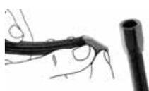
**Step 2.** Remove tape and then quickly insert hose into the socket. Insert hose with a turning motion, feeding the braid in as you turn the hose.
