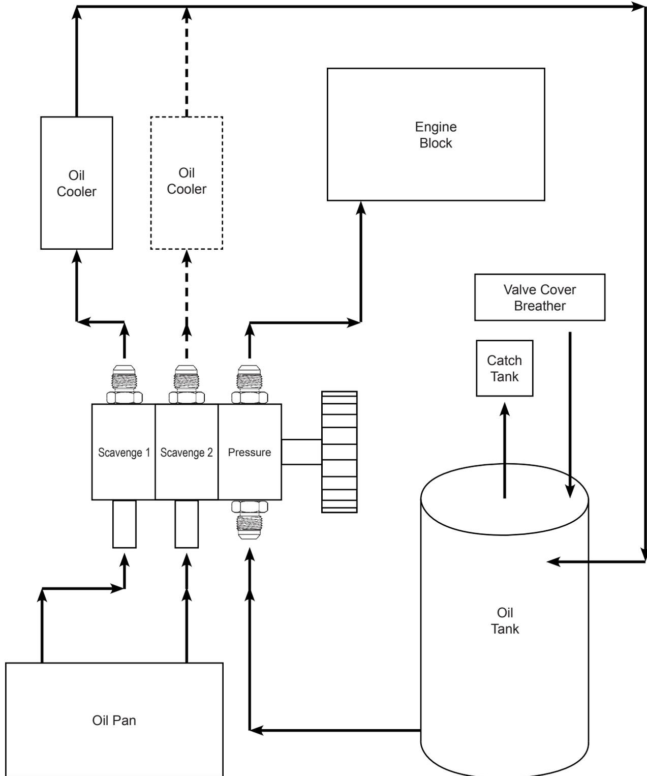
Note 1: Some pumps have outlets for each scavenge stage; others have only one outlet for both scavenge stages.
