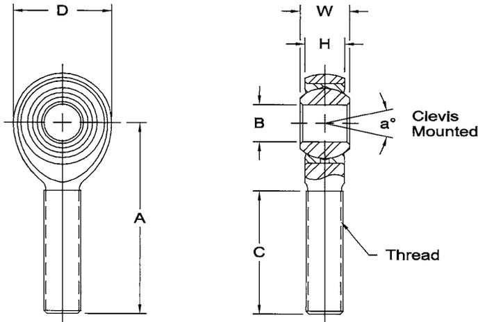
**Body:** Carbon steel, protective coated for corrosion resistance.
