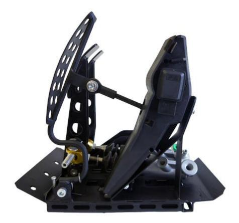
The Fly By Wire (FBW) unit is then bolted to the bracket on the E46 pedal box, you will need to drill the bracket and the FBW unit to secure.
