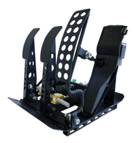
This is then fitted into the car using the floor pan angle to secure the pedal box.
