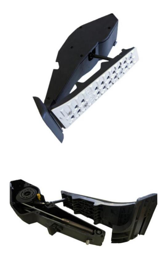
The first thing you will be required to do is remove the E46 Accelerator Pedal, remove the screws that hold the side cover on.
