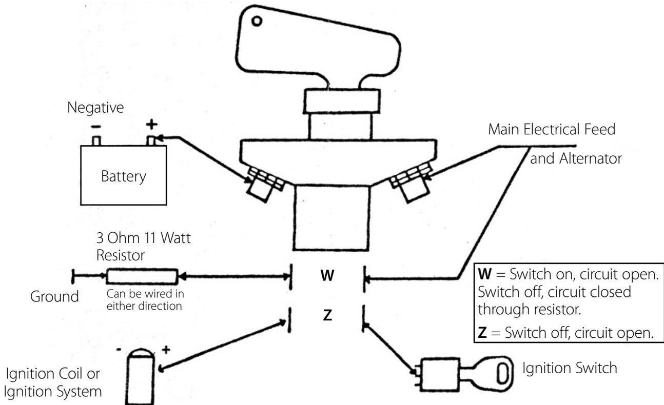
If you disconnect the battery while an alternator-equipped engine is running, the alternator could be damaged by a voltage spike. This spike can be avoided by giving the alternator output a safe path to ground just when the switch is turned off. Our 4430 Master Battery Switch has an auxiliary set of contacts (labeled "W") which are open when the switch is on, but which make contact when the switch is turned off.
