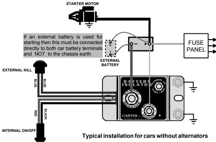
Typical installation for cars without alternators
