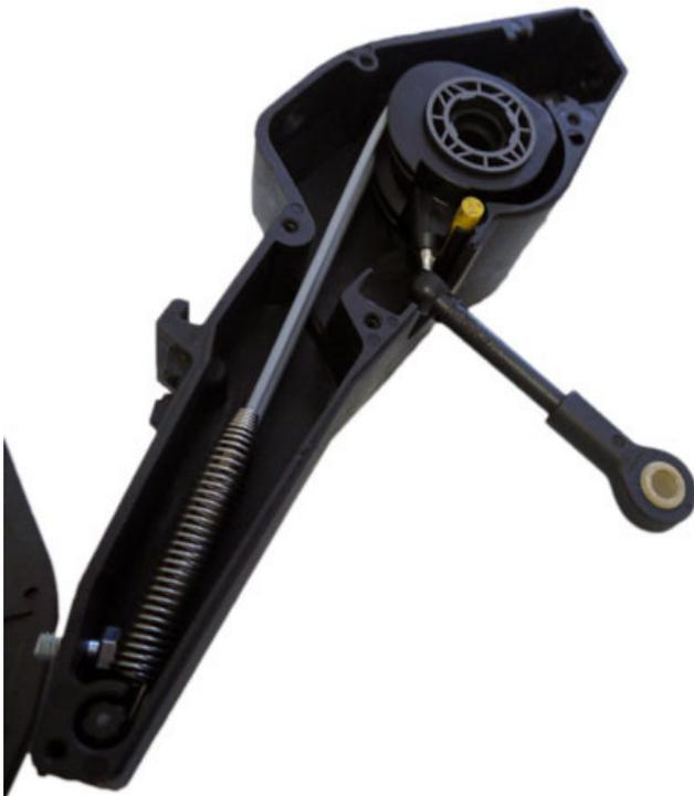
You will then have the pedal in the above state. You will need to cut the ball off the end of the push rod and connect the plastic ball joint that is supplied with the pedal box.
