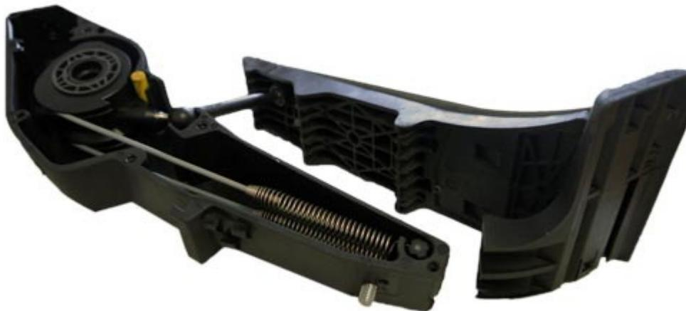
The first thing you will be required to do is remove the E46 Accelerator Pedal, remove the screws that hold the side cover on.
